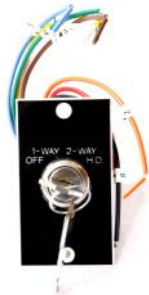
CM-DTMOD RF TRANSMITTER 318MHz FREQUENCY BOARD TRANSMITTER WIRES TO SWITCH
